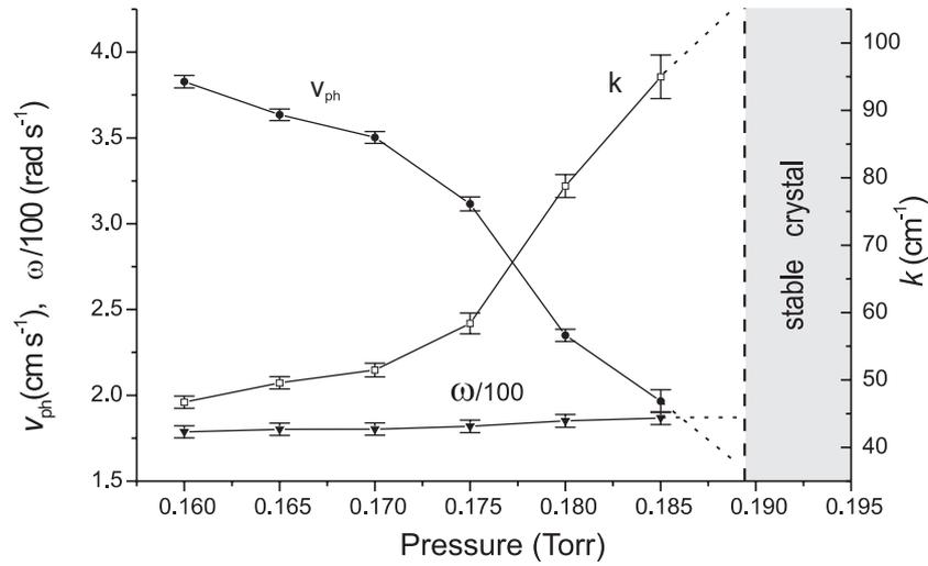
**Figure 3.** Dependence of the measured phase velocity,  $v_{\text{ph}}$ , and frequency,  $\omega$ , on the neutral gas pressure, below the critical pressure  $P_C = 0.188$  Torr. The wave number is calculated as  $k = \omega/v_{\text{ph}}$ .
